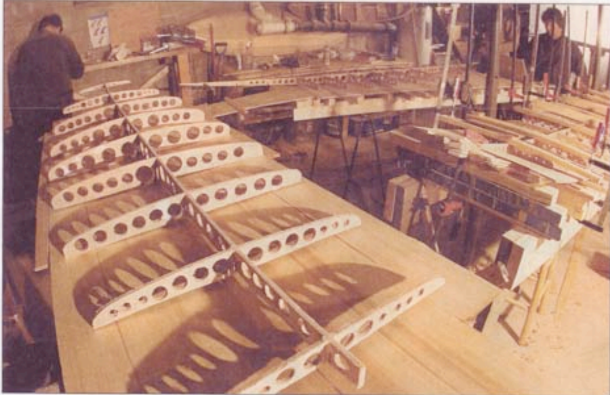
Board-building has much in common with the construction of other wooden watercraft: keel-mounted frames are skinned in planks of cedar and sheathed in fiberglass set in epoxy. Wooden boards weigh 20–30% more than foam-and-glass ones, but, says Rich Blundell, wood is “so beautiful.”
